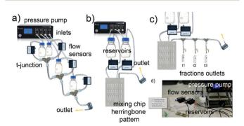
Fig. 1 Different microfluidic setups used for the reactions. Schematics of microfluidic setups with, (a) four asymmetrical inlets and T-junctions microfluidic reactor 1 (MR1), (b) two symmetrical inlets mixing chip microfluidic reactor 2 (MR2), (c) MR2 used for kinetics studies where the outlets for collection of reaction intermediates are also shown. (d) Picture of MR2
