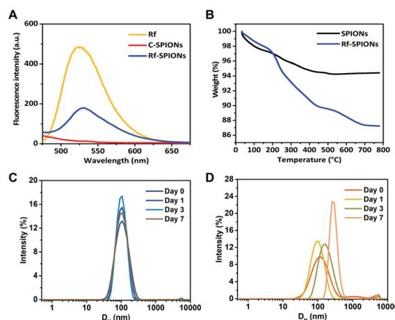
Fig. 4 (A) Fluorescence spectra ( $\lambda_{ex} = 440$  nm) of free Rf (yellow line), C-SPIONs (red line) and Rf-SPIONs (blue line). (B) Thermogravimetric curves of SPIONs (black line) and Rf-SPIONs (blue line). (C) Rf-SPION and (D) C-SPION DLS stability measurements.
