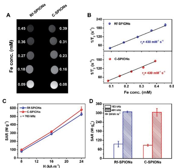
Fig. 6 (A)  $T_2$  weighted MR phantom image of the SPIONs. (B) Plot of  $T_2^{-1}$  versus Fe concentration for Rf-SPIONs (blue) and C-SPIONs (red) in water. (C) SAR values as a function of the applied magnetic field at a frequency of  $763 \text{ kHz}$  for the SPIONs. (D) SAR values of the SPIONs were measured at frequencies of  $163$  and  $491 \text{ kHz}$  under a constant magnetic field strength of  $24 \text{ kA m}^{-1}$ .
