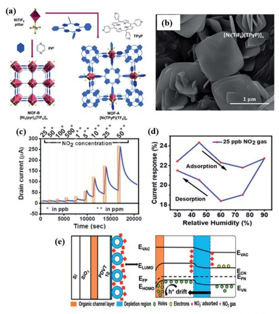
Fig. 22 (a) Schematic diagram of the preparation of the [Ni (TPyP)(TiF<sub>6</sub>)]<sub>n</sub> MOF, (b) SEM images of MOF-A [Ni(TPyP)(TiF<sub>6</sub>)]<sub>n</sub>, (c) sensing properties towards NO<sub>2</sub> gas, (d) humidity effect of the OFET gas sensor, and (e) sensing mechanism of PVDT-10 and MOF based OFET sensors. 177
