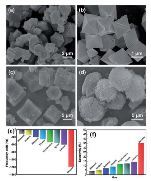
Fig. 20 FESEM images of the as prepared MOFs: (a) MOF-14, (b) HKAUST-1, (c) MOF-177, and (d) MOF-74, (e) response profile of the MOF-14based QCM sensor towards different VOCs for 100 ppm benzene at 25C°C, and (f) selectivity study of the MOF-14-sensor in different interfering gases towards 100 ppm benzene at RT. Reproduced from ref. 163 with permission from Elsevier, copyright 2021.
