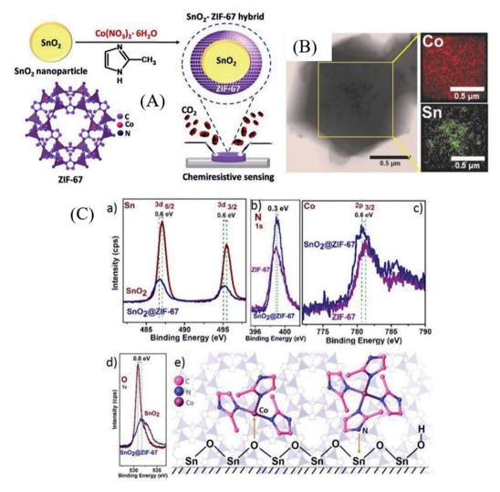
Fig. 9 (A) Schematic illustration of  $SnO_2@ZIF-67$  architecture formation, (B) TEM image of the core-shell  $SnO_2@ZIF-67$  material with its corresponding EDX-elemental analysis, and (C) XPS analysis to examine the synergistic effect of  $SnO_2$  and the ZIIF-67 MOF. Reproduced from ref. 101 with permission from Wiley-VCH GmbH, copyright 2021.
