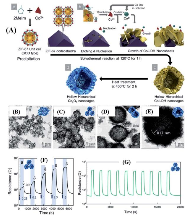
Fig. 6 (A) Synthesis protocol of hierarchical hollow  $Co_3O_4$  nanocages using ZIF-67 as the template, (B–E) SEM images of  $Co_3O_4$  hierarchical hollow nanocages (HHN) with different sizes, (F) response/recovery curves of the  $10-\text{Co}_3\text{O}_4$  sensor tested at  $225\,^{\circ}\text{C}$  towards p-xylene (0.5–2.5). ppm), and (G) repeatability test at 225 °C. Reprinted from ref. 88 with permission from American Chemical Society, copyright 2021.
