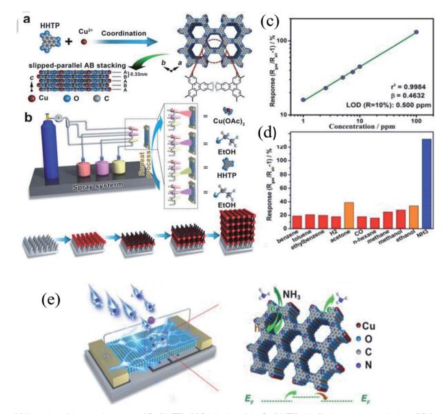
Fig. 3 (a) Illustration of the crystal structure of Cu<sub>3</sub>(HHTP)<sub>2</sub>. (b) Fabrication of the Cu<sub>3</sub>(HHTP)<sub>2</sub> thin film by a spray layer-by-layer (LBL) method using the LPE technique, (c) LOD graph, (d) selectivity test of the  $Cu_3(HHTP)_2$  thin-film sensor, and (e)  $NH_3$  sensing mechanism of the  $Cu_3(HHTP)_2$ thin film sensor at RT. Reproduced from ref. 70 with permission from Wiley Sons, copyright 2021.
