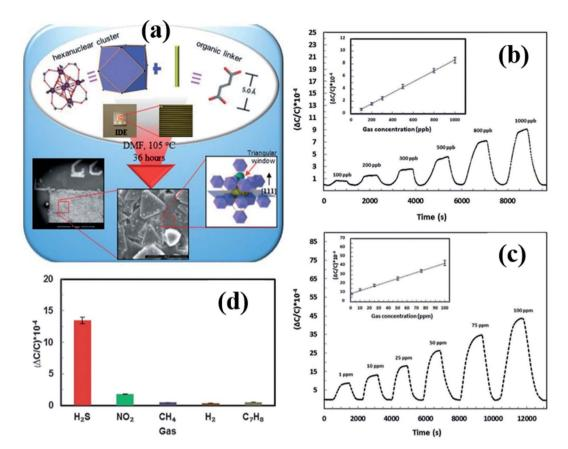
Fig. 16 (a) The schematic diagram of the preparation of the fum-fcu-MOF by the solvothermal method and its integration onto the IDE, (b and c) capacitive response transients of the fum-fcu-MOF sensor for the ppb and ppm levels of  $H_2S$  detection, and (d) the selectivity test of the fum-fcu-MOF sensor towards different interfering gases. Reprinted from ref. 137, copyright@2021, Wiley and Sons.
