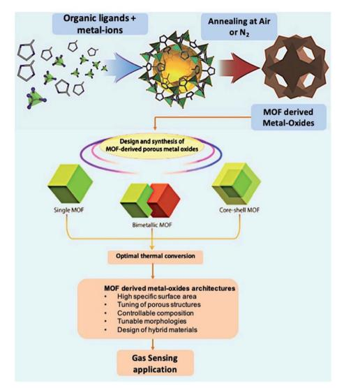
Fig. 5 Graphical representation of the preparation of MOFs and MOF-derived metal-oxide structures and their structural and morphological advantages for gas sensing applications. Adopted from ref. 77 with permission from American Chemical Society, copyright 2021.
