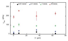
**Fig. 4** Effect of elastomer thickness on ice adhesion in shear mode test.  $\tau_{\rm ice}$  remains independent of the elastomer thickness, h, at different shear velocities and a surface temperature,  $T=-20~{\rm ^{\circ}C}$ . Error bars represent standard deviation for  $n_{\rm e}\geq 3$  independent experiments.
