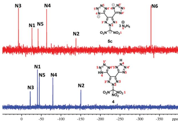
Fig. 2 <sup>15</sup>N NMR spectra of **4** and **5c**.
