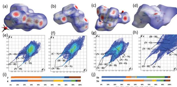
Fig. 10 Hirshfeld surface calculations (a–d), and 2D fingerprint plots (e–h) of the crystal structures **4**, **7**, **5a-H<sub>2</sub>O**, and **5b-H<sub>2</sub>O**. Populations of individual contacts for **4-MeOH**, **7** (i), and **5a-H<sub>2</sub>O**, **5b-H<sub>2</sub>O** (j).
