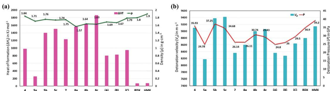
Fig. 8 Calculated heats of formation, experimental densities (a), calculated detonation velocities, and detonation pressures (b) of **4**, **5a–c**, **7**, **8a–c**, and compared with those of **A**, **B**, **C**, **RDX**, and **HMX**.
