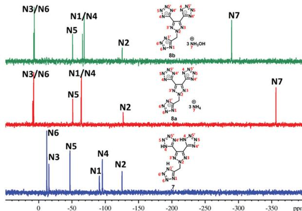
Fig. 3 <sup>15</sup>N NMR spectra of **7**, **8a** and **8b**.
