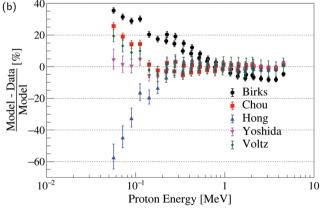
Fig. 3 (a) Specific luminescence models applied to EJ-204 proton light yield data from Laplace et al. 11 (b) Percent difference of the measured data with respect to the model prediction. The error bars represent the 68.27% confidence interval
