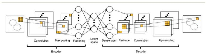
Fig. 2 Encoding-decoding layout of the constructed CAE
