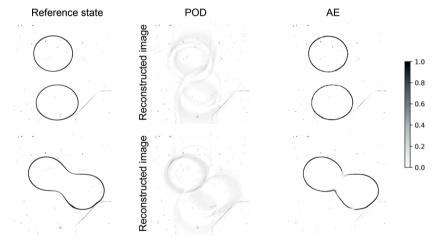
(a) Reconstructed image of drops entering the mixing chamber ( $140^{th}$ ) and the coalescence ( $651^{st}$ ). The time interval between sequential frames is 1 ms
