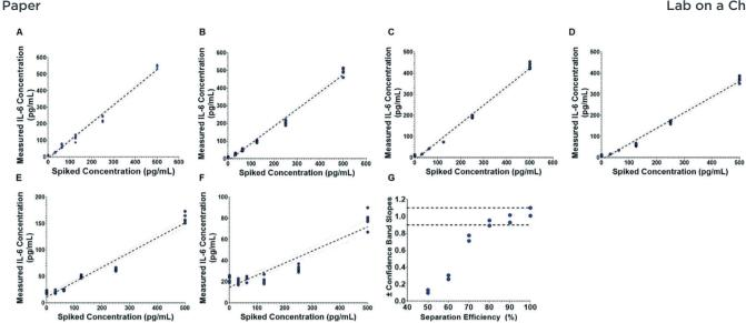
Fig. 6 Comparison of biosensor IL-6 measurements (n = 5) to theoretical spiked concentrations plasma separation efficiencies of (A) 99.98%, (B) 90, (C) 80%, (D) 70%, (E) 60% and (F) 50%. The dotted lines show the linear regression and 95% confidence bands. (G) Shows the variation from linearity
