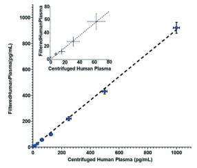
Fig. 3 ELISA measurements of spiked IL-6 concentrations for samples suspended in human plasma vs. samples which were filtered using the Vivid membrane from IL-6 spiked whole blood to plasma at 50  $\mu$ l min<sup>-1</sup> infusion rate. Inset shows results at lower concentrations. Dotted line represents a linear curve fit of y = 0.91x with an  $R^2$  value of 0.95.
