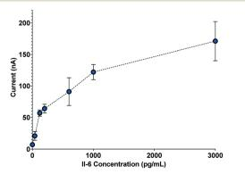
4 Sample amperometry measurement curve depicting electrochemical measurements from five separate biosensors.
