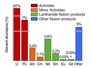
Fig. 1 Relative abundance of the actinides and lanthanide fission products in the spent MOX fuel sample used in this study, as calculated by neutronics computer codes. Line breaks are present for the highly abundant U and Pu and for the group of other fission products.
