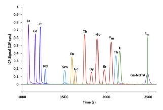
Fig. 2 Electropherogram obtained by CE-Q-ICP-MS for the mixture containing 14 lanthanides, uranium and thorium with a 100 mmol L $^{-1}$   $\alpha$ -HMBA electrolyte. Here,  $t_{\rm eo}$  is the time where neutrals migrate, as calculated at the apex of the Ga–NOTA peak. Yb and Lu were omitted from the figure for visibility reasons.
