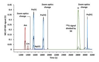
**Fig. 6** Electropherogram obtained by CE-MC-ICP-MS for actinides in a spent MOX fuel sample with a 120 mmol L $^{-1}$   $\alpha$ -HMBA electrolyte. The line breaks were caused by the change in zoom optics during the CE separation.
