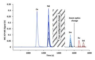
Fig. 7 Electropherogram obtained by CE-MC-ICP-MS for lanthanide fission products in a spent MOX fuel sample with a 120 mmol  $\rm L^{-1}$   $\alpha$ -HMBA electrolyte. The signal break between 1300 and 1500 s was caused by a cup configuration change, while the shorter signal break between 1575 and 1625 s was due to a modification in zoom optics.
