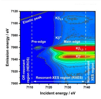
Fig. 1 RXES plane of FeCl<sub>3</sub> with all important features and HEROS, RXES, and nXES regions marked.
