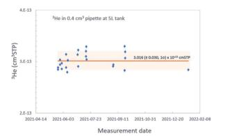
Fig. 5 An example of calibration results of the  $^{3}$ He amount in one of the pipettes. Solid line showing the average of all calibration results (n = 23) and shaded band signifying 2 sigma errors are shown.
