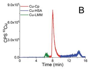
Fig. 5 Chromatograms of separation of the 15-times diluted human serum samples (A) H5 and (B) H1 on the CLC monolithic column monitored by ICP-MS detection at m/z 63.
