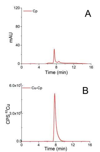
Fig. 3 Chromatograms of separation of the 15-times diluted sample of the standard serum protein Cp (3 g  $\rm L^{-1}$ ) on the CLC monolithic column monitored by (A) UV detection (278 nm) and (B) ICP-MS detection at m/z 63.
