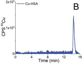
Fig. 2 Chromatograms of separation of the 15-times diluted sample of the standard serum protein HSA (25 g  $L^{-1}$ ) on the CLC monolithic column monitored by (A) UV detection (278 nm) and (B) ICP-MS detection at m/z 63.
