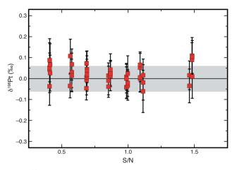
Fig. 5  $\,\delta^{198}$ Pt values of IRMM-010 Pt standard solutions with variable ratios of spike-derived Pt to natural Pt (S/N). The solutions were analysed relative to a solution with S/N = 0.84. The grey shaded area represents the typical between-run precision of the bracketing standard solutions. For solutions with S/N = 0.7 to 1.0, the uncertainties in  $\delta^{198}$ Pt are a factor of  $\sim$ 1.5 better than for solutions with S/N outside this range.
