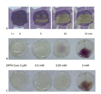
**Fig. 4** (A) **5P-17** spotted onto cotton fabric soaked with DPPH (purple, 5 mM) in IPA; time lapse over 5 minutes showing both antioxidant activity and diffusion of oil through the fabric. (B) From left to right, 5  $\mu$ M, 0.05 mM, 0.5 mM, and, 5 mM DPPH in IPA solution spotted onto **5E-75** t=15 s, (C) t=90 s.
