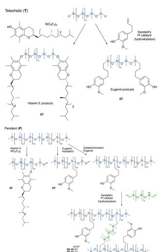
Fig. 2 Preparation of antioxidant-modified silicones.
