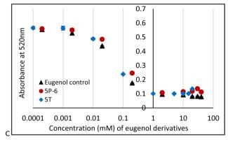
Fig. 3 Log plots of DPPH UV assay at 520 nm wavelength, comparison of anti-oxidation activity of: (A) retinoic acid, homoallyl retinoate and silicone derivatives 3T and 3P-6; (B) tocopherol, tocopheryl acetate, and silicone adduct 4T; (C) eugenol and eugenol-modified silicones 5T and 5P-6. Error bars reflect the standard error of 3 UV measurement trials.
