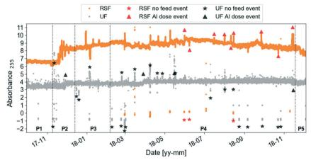
Fig. 4 Same preprocessed UV absorbance at 255 nm (absorbance per meter) time-series as in Fig. 2 (zoomed out) with two types of events labelled by the user using the function *outlier\_id\_drop* in the AbspectroscoPY toolbox for rapid sand filtrate (RSF) and ultrafilter permeate (UF). The symbol identifies the whole event period, using the average timestamp of the event as *x*-axis coordinate and the median absorbance value at 255 nm plus-minus one absorbance unit offset as *y*-axis coordinate.
