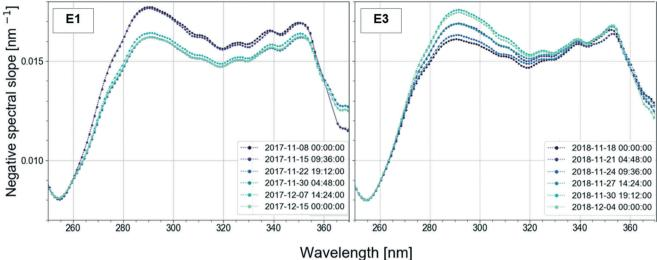
Fig. 5 Spectral slope curve of the spectro::lyser absorbance data in surface water as a function of wavelength calculated using the abs\_spectral\_curve function in the AbspectroscoPY toolbox. The selected dates cover the period before, during and after the autumn lake circulation event in 2017 (left plot, November-December, event 1) and 2018 (right plot, November-December, event 3).
