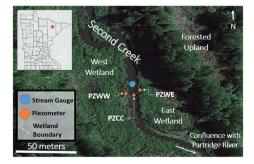
Fig. 1 Second Creek study area showing the stream channel and riparian wetlands in northeastern Minnesota (inset) with the specific locations of groundwater piezometers (orange circles), stream gauge (blue circle) and wetland boundaries (white dashed lines). Samples for sediment and aqueous geochemistry were taken adjacent to the piezometers for the west wetland (PZWW), east wetland (PZEW), and stream channel center (PZCC). This figure is based on Fig. 1 in Ng et al. (2017).
