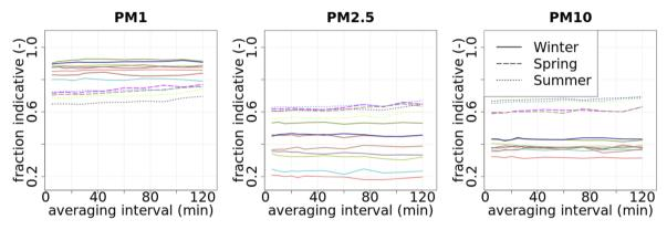
Fig. 7 Fraction of indicative LCS uncalibrated measurements as a function of the averaging time (minutes). Each color represents an individual system/campaign pair. The line style indicates the campaign: winter (solid lines), spring (dashed lines) and summer (dotted lines).
