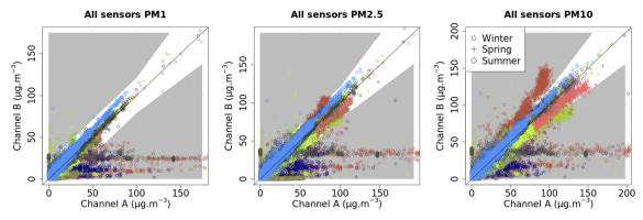
Fig. 1 Inter-channel performance of the PurpleAir systems for  $PM_1$ ,  $PM_{2.5}$  and  $PM_{10}$  (1 minute readings). Each color represents an individual system/campaign pair. The shaded areas represent measurements that do not meet the QA/QC criteria.
