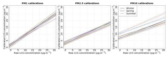
Fig. 3 Linear calibration of the LCS PM measurements. Each color represents an individual LCS/campaign pair. Line styles distinguish the campaigns: winter (solid lines), spring (dashed lines) and summer (dotted lines).
