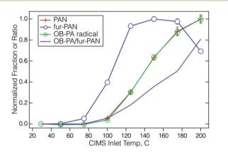
Fig. 3 The temperature profiles of the I $^-$  CIMS response to PAN and fur-PAN plotted relative to their highest signal, along with the signal at m/z 99 tentatively assigned to OB-PAN.
