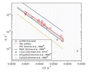
Fig. 6 Arrhenius plot of the thermal decomposition of fur-PAN compared to a number of other acyl peroxynitrate compounds. The individual data points are shown as open circles, with error bars for individual data points, and the fit to the Arrhenius expression is shown as a solid red line. Examples of other Arrhenius expressions are given as noted in the legend, with either the common acronym, or acyl radical, specified.
