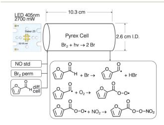
Fig. 1 Schematic of the fur-PAN photochemical source and associated chemistry.
