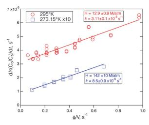
Fig. 7 The results of Henry's law coefficient measurements in DI  $H_2O$  at 295 K, and 273.15 K (enlarged  $\times 10$  on the y-axis). The errors in individual decay rates are smaller than the width of the symbols. The H and K values and associated uncertainties were obtained from the fit of the data points to eqn (3).
