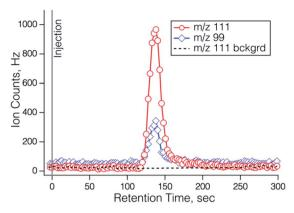
Fig. 4 GC trace during the separation of the effluent of the fur-PAN source on a 2 m Rtx-1 column, 0.53 mm ID, 1.5  $\mu$ m film thickness. The furoate anion (m/z 111) is shown in red and the 4-oxo-2-butenoate anion (m/z 99) is shown in blue
