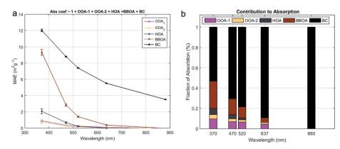
Fig. 8 (a) Mass absorption efficiencies (MAE) for each component (OA factors and BC), and MAEs are the coefficients from multivariate linear regression. The error bars represent the coefficient standard deviation and (b) estimate of the contribution of OA and BC to the absorption coefficient at each wavelength.
