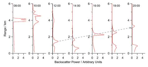
Fig. 10 MiniMPL range corrected co-polarisation normalised relative backscatter signal above Brighton and Hove on the 16<sup>th</sup> October 2017 at 2-hourly intervals between 08:00 and 20:00 UTC. The grey dashed arrow shows the base of the optically dense layer rising throughout the afternoon.
