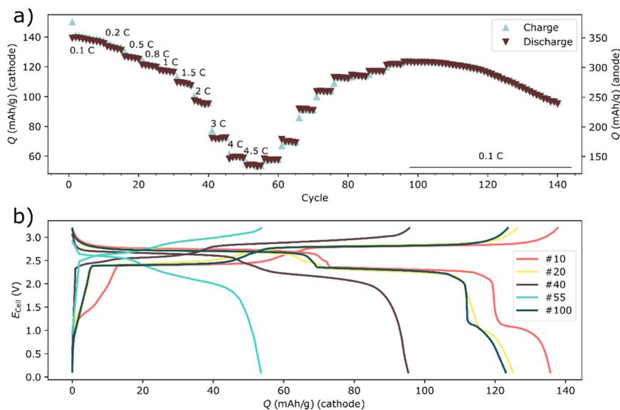
**Fig. 4** The rate test of a two-electrode Prussian white – Bismuth full-cell. The discharge retention during the symmetrical rate test is shown in a for cycles 1–140, whereas the voltage profile for selected cycles are shown in (b). The indicated C rates in (a) are based on the capacity of the anode. The current densities for the cycles in (b) are shown in Table S1.†
