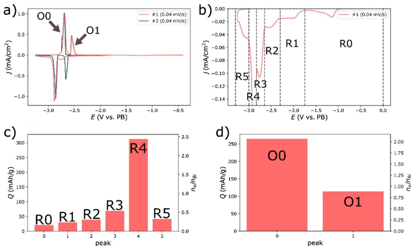
**Fig. 2** (a) The initial two cycles during a cyclic voltammetry measurement. (b) The first reduction sweep of bismuth. The notation indicates the index of each peak-domain during reduction (R#) and oxidation (O#) respectively. The capacity for each domain is shown for the reduction in (c) and oxidation in (d).
