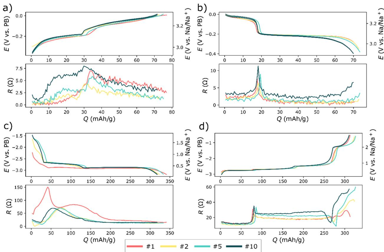
**Fig. 7** Three-electrode ICI measurements using Prussian white cathode, bismuth anode, and Prussian white reference electrode. The voltage profile and coinciding resistances are shown for the Prussian white cathode for charges (a) and discharges (b). Similarly, (c) and (d) show the potential and resistance on the anode during charging (c) and discharging (d).
