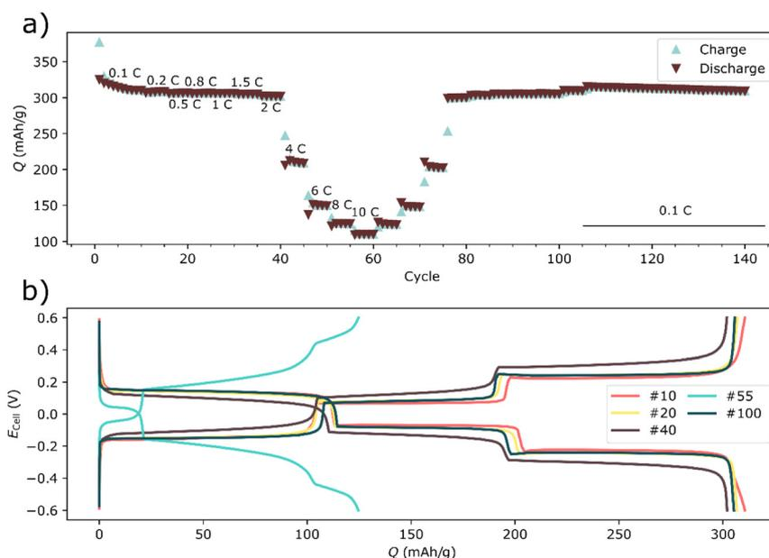
**Fig. 5** The rate test of a two-electrode bismuth symmetrical cell. The discharge retention during the symmetrical rate test is shown in a for cycles 1–140, whereas the voltage profile for selected cycles are shown in (b). The current densities for the cycles in (b) are shown in Table S2.†
