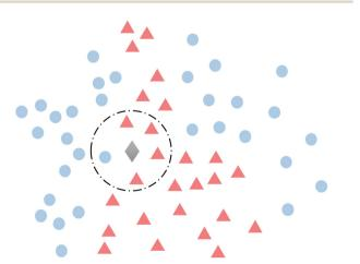
Fig. 5 A simple example of the kNN algorithm approach. The blue dots and red triangles represent the training instances with two labels, and the grey diamond is a new test instance. In this example k is set as 5, and the 5 nearest instances are included in the black circle. As there are 4 red triangles and only 1 blue dot, the class of the test instance is classified as a red triangle.
