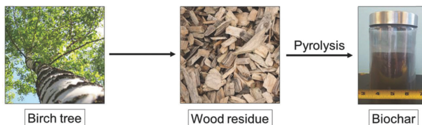
Fig. 62 Schematic representation of biochar formation. Reproduced with permission from ref. 1002. Copyright Wiley 2018.
