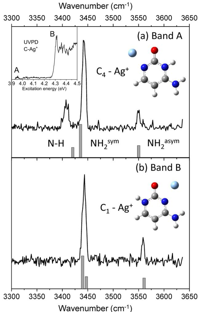
Fig. 1 Observed and calculated IR spectra of the C–Ag<sup>+</sup> complex with the UV wavelength set on (a) the band A at 3.95 eV and (b) the band B at 4.32 eV. The UVPD spectrum of C–Ag<sup>+</sup> is reported in insert with the 2 UV transitions labeled A and B used for producing the cytosine radical cation.
