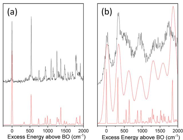
**Fig. 5** Comparison between the experimental and FC simulations of (a) the  $D_0$ – $D_4$  transition of  $C_1^{\bullet+}$  and (b) the  $D_0$ – $D_3$  transition of  $C_4^{\bullet+}$ . Calculated frequencies (UCAM-B3LYP/aug-cc-pVDZ) scaled by 0.95. BO is for “Band Origin”.
