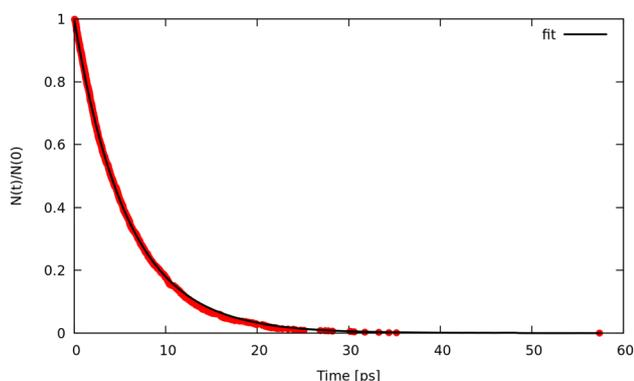
Fig. 5 Population decay obtained from RPMD simulations with  $\gamma = 0.01$  fs<sup>-1</sup>,  $P = 8$  and  $T = 4500$  K using Potential C. Red dots are the simulation data, black solid line corresponds to a single-exponential fit.
