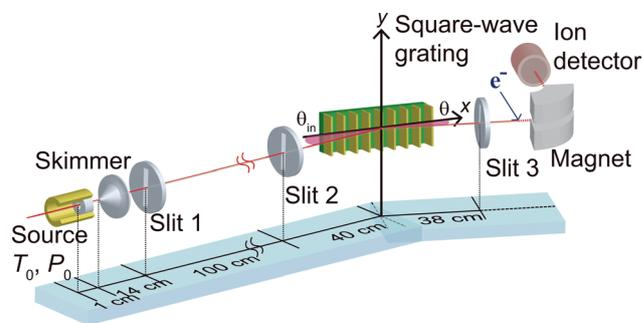
**Fig. 2** Schematic of the experimental setup used for reflection of He molecular beams from square-wave gratings. The illustration shows the definitions of the incidence angle  $\theta_{\text{in}}$  and detection angle  $\theta$ .
