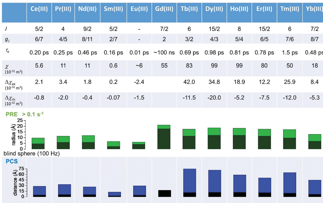
Fig. 2 Typical values of electron relaxation time ( \tau_e ), magnetic susceptibility ( \chi ) and axial and rhombic anisotropy ( \Delta\chi_{ax} and \Delta\chi_{rh} ) of lanthanoid ions. The typical radii of blind spheres (black) and spheres with ^1\text{H} PREs larger than 0.1 \text{ s}^{-1} (green), and the maximum distances of nuclei in axial position with PCSs of 0.05 \text{ ppm} (blue) are also shown for a protein with the reorientation time of 10 \text{ ns} at 700 \text{ MHz} .
