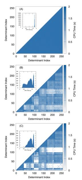
Fig. 6 Heat maps of the time to compute each of the two electron terms (CPU time) with respect to the determinant index using the unscaled density (A) vs. the overlap-scaled density algorithm (B) and the overlapscaled density with the Slater-Condon screening (C). A histogram of each set of timings (summed over all respective elements) are included in the inset.
