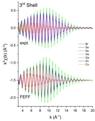
**Fig. 10** Third-shell, single-scattering contributions to the EXAFS shown in Fig. 3 compared to their FEFF simulations. The FEFF simulations include  $\sigma^2$ , but not  $S_0^2$  or  $E_0$  corrections (see text).
