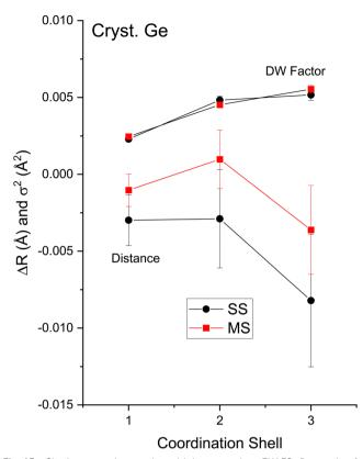
Fig. 15 Single-scattering and multiple-scattering EXAFS fit results for crystalline Ge. The figure plots changes in bond lengths  $\Delta R_{1.2.3}$ and Debye-Waller factors  $\sigma_{1,2,3}^{2}$  for the first-, second-, and thirdcoordination shells. Results of single-scattering (black) and multiplescattering (red) fits are indicated (see text).
