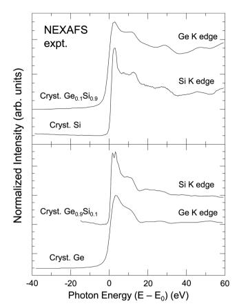
Fig. 2 Sensitivity of XAFS to backscattering environment. Top: Si K edge of crystalline Si and Ge K edge of a dilute Ge in Si crystalline Ge<sub>0.1</sub>Si<sub>0.9</sub> alloy. Bottom: Ge K edge of crystalline Ge and Si K edge of a dilute Si in Ge crystalline Ge<sub>0.9</sub>Si<sub>0.1</sub> alloy. The splitting of the white line (or "rabbit ears") observed at the Si K edge is a density of states effect (see text). (After Woicik and Pianetta. 10)
