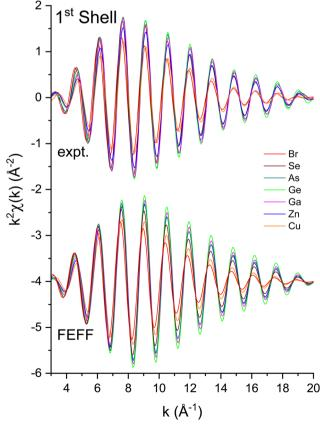
Fig. 8 First-shell, single-scattering contributions to the EXAFS shown in Fig. 3 compared to their FEFF simulations. The FEFF simulations include  $\sigma^2$ , but not  $S_0^2$  or  $E_0$  corrections (see text).
