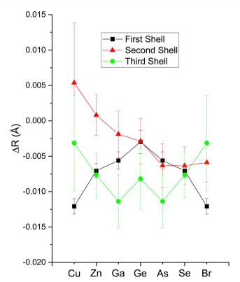
Fig. 17 EXAFS fitting results for crystalline CuBr, ZnSe, GaAs, and Ge at the Cu, Zn, Ga, Ge, As, Se, and Br K edges as indicated. Both edges of each heteropolar material were co-refined. The figure plots changes in the first-, second-, and third-shell bond lengths  $\Delta R_{1,2,3}$  from their room-temperature values (see text).
