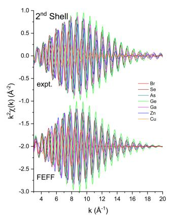
**Fig. 9** Second-shell, single-scattering contributions to the EXAFS shown in Fig. 3 compared to their FEFF simulations. The FEFF simulations include  $\sigma^2$ , but not  $S_0^2$  or  $E_0$  corrections (see text).
