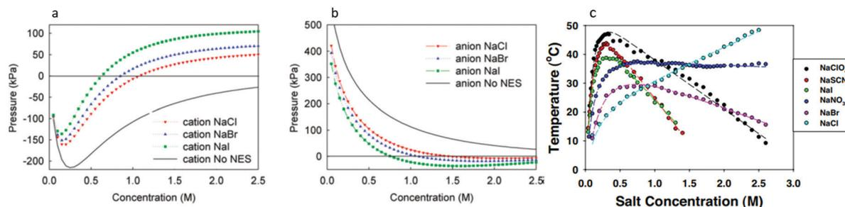
**Fig. 5** The salt concentration dependence of the double-layer pressure between two surfaces separated by 20 Å showing separate (a) anion and (b) cation influences.<sup>172</sup> (c) The cloud-point temperature of lysozyme as a function of anion type and concentration.<sup>25</sup> (a) and (b) reprinted from ref. 172 with permission from the American Chemical Society, copyright 2011. (c) Reprinted from ref. 25 with permission from the National Academy of Sciences, copyright 2009.
