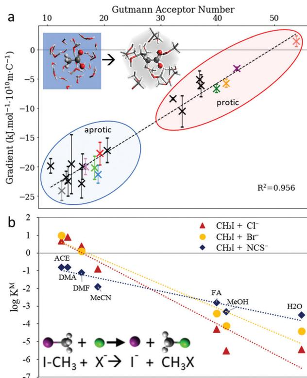
Fig. 15 The Gutmann acceptor number approximates the effect of the solvent on anion trends (a) with the Gibbs' free energy of transfer from aqueous to nonaqueous solvents and (b) the  $S_N2$  reaction rate with methyl iodide. Adapted from ref. 128 with permission from the Royal Society of Chemistry, copyright 2021.
