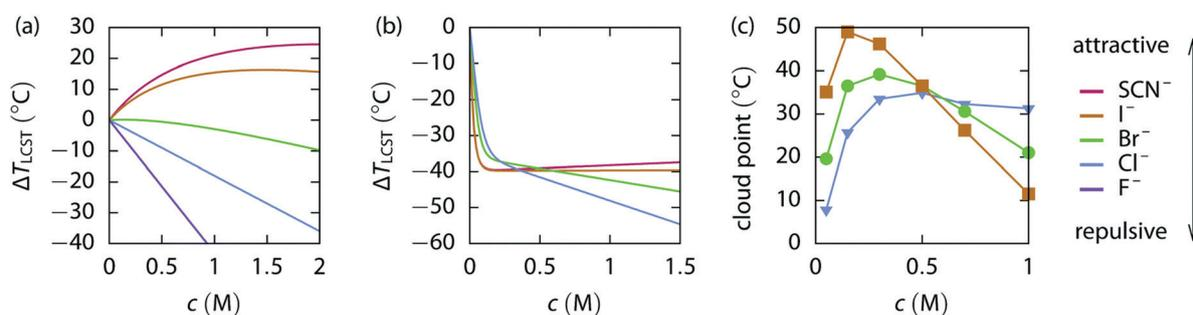
Fig. 6 LCST change vs. the concentration of various sodium salts for (a) uncharged ELP V<sub>5</sub>A<sub>2</sub>G<sub>3</sub>-120, (b) weakly positive ELP KV<sub>6</sub>-112 and (c) the UCST for weakly positive PAU.<sup>177</sup> Reproduced from ref. 177 with permission from the Royal Society of Chemistry, copyright 2018.
