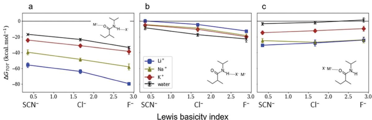
Fig. 9 GKS-EDA (M062X/cc-pVDZ) interaction energies between (a) dissociated salts and associated salts at (b) the N–H and (c) the C=O sites of a NIPAM monomer in water. Black atoms in the inset structures indicate GKS-EDA fragments considered. All data is the average of 10 independent configurations; error bars denote 1 standard deviation. Reprinted with permission from ref. 45 with permission from the American Chemical Society, copyright 2019.
