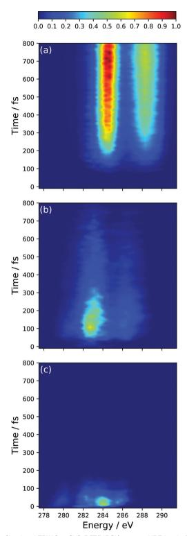
Fig. 6 Simulated TRXAS at CVS-DFT/MRCI/aug-cc-pVDZ level of theory, decomposed into contributions from the (a)  $S_0$ , (b)  $S_1$  and (c)  $S_2$  adiabatic states.
