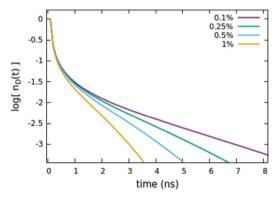
Fig. 7 Effect of the quencher concentration  $C_q$  (expressed as % of  $C_d^{TOT}$ ) on the (normalized) exciton density decay. Fixed parameters are  $R_{d^*d} = 5 \text{ nm}$ ;  $R_{d^*d^*} = 4 \text{ nm}$ ;  $R_{d^*q} = 2 \text{ nm}$ ;  $\tau_q = 4 \text{ ns}$ ,  $C_q = 0.25\%$  of  $C_d^{TOT}$ ;  $n_{d}(0) = 7\% \text{ of } C_{d}^{TOT}$
