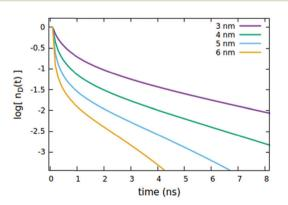
Fig. 5 Effect of the  $R_{d*d}$  radius governing both EEA and quenching diffusive mechanisms on the (normalized) exciton density decay. Fixed parameters are  $R_{d^*d^*} = 4$  nm;  $R_{d^*q} = 2$  nm;  $\tau_q = 4$  ns;  $C_q = 0.25\%$  of  $C_d^{TOT}$ ;  $n_{\rm d}(0) = 7\% \text{ of } C_{\rm d}^{\rm TOT}$
