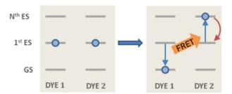
Fig. 1 The mechanism for exciton-exction annihilation (EEA). The excitation is transferred between two excited dyes (DYES 1 and 2), leading to an excited state absorption (to the Nth excited state) in one dye (DYE 2) and to a relaxation to the ground state in the other one (DYE 1). The Nth highlying state is expected to rapidly decay non-radiatively (red arrow) to the first excited state, leading to the annihilation of one excitation (i.e. that of DYE 1).
