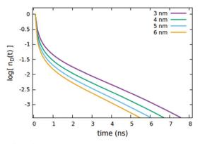
Fig. 4 Effect of the  $R_{d^*d^*}$  radius governing the direct EEA mechanism on the (normalized) exciton density decay. Fixed parameters are  $R_{d^*d} = 5$  nm;  $R_{d*q} = 2 \text{ nm}; \ \tau_q = 4 \text{ ns}; \ C_q = 0.25\% \text{ of } C_d^{TOT}; \ n_d(0) = 7\% \text{ of } C_d^{TO}$
