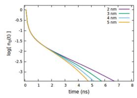
Fig. 6 Effect of the  $R_{d*q}$  radius governing the direct quenching mechanism on the (normalized) exciton density decay. Fixed parameters are  $R_{d^*d^*} = 4 \text{ nm}$ ;  $R_{d^*d} = 5 \text{ nm}$ ;  $\tau_q = 4 \text{ ns}$ ;  $C_q = 0.25\%$  of  $C_d^{TOT}$ ;  $n_d(0) = 7\%$  of  $C_d^{TOT}$ .
