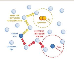
Fig. 3 The two possible mechanisms for the exciton loss in the presence of both EEA and quenching species (such as dimers in the case of rhodamine B) described by the Gösele model in the predominant direct mechanism regime. The new introduced contact radii  $R_{\rm EEA}$  and  $R_{\rm q}$  depend on the Förster radii  $R_{\rm d^*d^*}$  and  $R_{\rm d^*q}$  respectively, and also depend on the same diffusion coefficient D.
