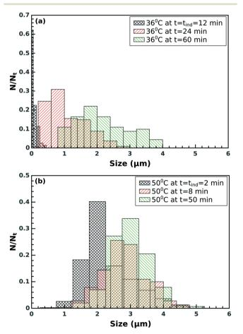
Fig. 6 Particle size distribution (a) at 36  $^{\circ}$ C and (b) at 50  $^{\circ}$ C at different times for flat-sheet-like crystals.
