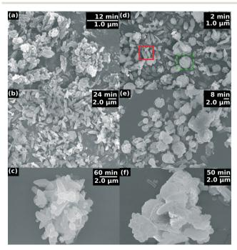
Fig. 5 SEM images of particles obtained at different temperatures and at different crystallization times: (a–c) 36 °C, (d–f) 50 °C with  $[Na_3PO_4]_0$  = 0.030 M and R = 3. The red box indicates a fully developed flat-sheet-like crystal, while the green dashed box a floral shaped crystal from aggregation.
