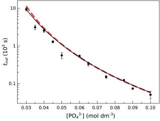
Fig. 2 Induction time as a function of initial phosphate concentration at T = 25 °C. The black solid line shows the power-law fitting according to egn (1). The red dashed line represents the calculated induction times from the kinetic model based on eqn (9)-(13).
