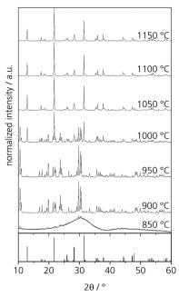
Fig. 5 XRD patterns of glass ZrO after heat treatments for 5 h at different temperatures. The theoretical peaks displayed at the bottom are attributed to NaYSi<sub>2</sub>O<sub>6</sub> (calculated from ICSD 171255, ref. 16).
