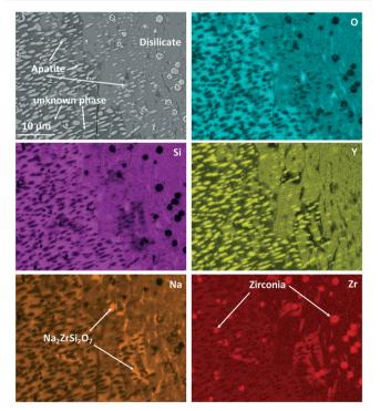
Fig. 10 EDXS elemental mapping of Zr9 after a two-step heat treatment at 820 °C for 20 h + 1150 °C for 1 h. The mapping was recorded in the area of Fig. 9 marked with "EDXS".
