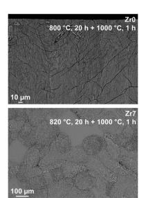
Fig. 7 SEM micrographs of glasses Zr0 and Zr7 after two-step heat treatments at 820 °C for 20 h and 1000 °C for 1 h.
