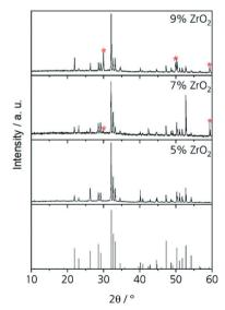
Fig. 3 XRD patterns of Zr5, Zr7, Zr9 and Zr11 after slow cooling to room temperature. The theoretic pattern at the bottom belongs to NaY<sub>9</sub>Si<sub>6</sub>O<sub>26</sub> (JCPDS no. 00-035-0404). The peaks of cubic zirconia (JCPDS no. 01-077-2112) are marked with red stars.
