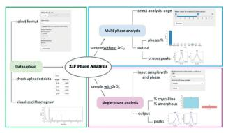
Fig. 4 Workflow of the ZIF Phase Analysis app
