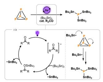
Scheme 2 Proposed mechanism for the light-driven, photocatalytic stannylation of P<sub>4</sub> in the presence of hexabutyldistannane, (Bu<sub>3</sub>Sn)<sub>2</sub>, and a ketone photocatalyst, R2CO
