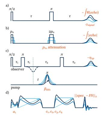
Fig. 2 Schematic representations of pulse sequences and elements subjected to optimisations: (a) phase of the detected signal after a Hahn echo, (b) flip angles of 90° and 180° pulses of a Hahn echo, parametrized by pulse length and amplitude, (c) The HS pump pulse in a 4-pulse DEER experiment, and (d) pulse waveforms in the CHORUS sequence. Parameters subjected to the optimisation and their corresponding cost function are indicated in orange, respectively, below and above each sequence.
