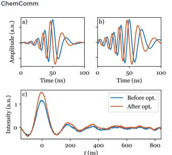
Fig. 3 Cartesian representation of the HS pump pulse in a 4-pulse DEER experiment, (a) before ( $\beta$  = 10), and (b) after ( $\beta$  = 6) optimisation, with (c) corresponding full DEER traces for bisnitroxide (Scheme 1).
