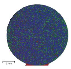
Fig. 6 A LDIR chemical image of a full single tablet of pharmaceutical formulation, where blue = microcrystalline cellulose, green = lactose monohydrate, red = hydrobromide salt API and magenta = croscarmellose sodium.
