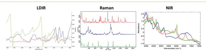
Fig. 1 The LDIR (left), Raman (centre) and NIR (right) spectra of hydrobromide salt API (red), microcrystalline cellulose (blue) and saccharin (green).
