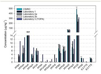
Fig. 3 Interlaboratory comparison of PFAS concentrations in an asphalt core (Core 6 top 50 mm). CSIRO, Laboratory 1 and Laboratory 2a conducted the sample extraction and analysis independently. The extracts at CSIRO were also analysed by Laboratory 2 (represented as Laboratory 2b). Laboratory 3 only conducted total oxidisable precursor assay (TOPA).
