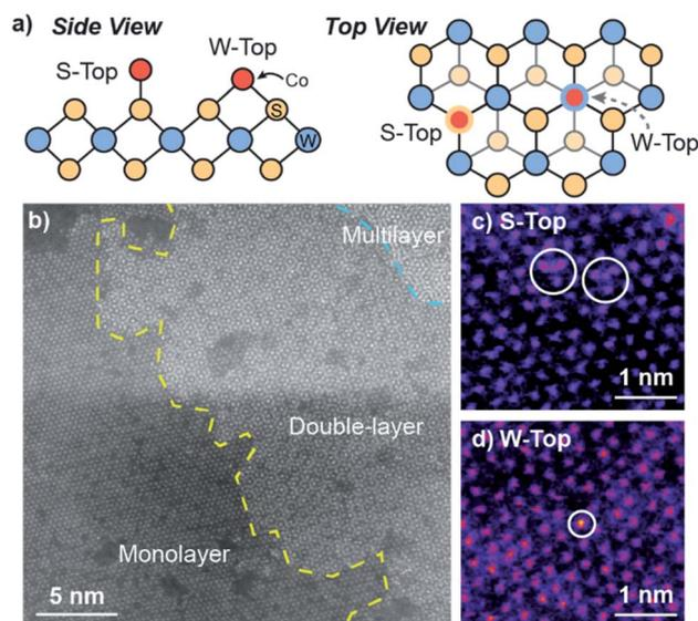
**Fig. 1** (a) Schematic depicting side and top views for S-top and W-top binding of Co atoms on WS<sub>2</sub>, (b) high-resolution STEM image of colloidal 0.3Co-WS<sub>2</sub>, (c) HR-STEM region containing S-top Co sites, and (d) HR-STEM region containing W-top sites.
