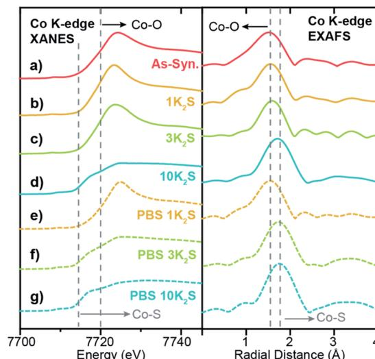
Fig. 6 Co K-edge XANES and EXAFS spectra for 1.0Co-WS<sub>2</sub> samples at varying stages of synthesis and catalysis. (a) As-synthesized, (b–d) thermally treated with varying equivalents of K<sub>2</sub>S, and (e–g) immersed in 1 M PBS electrolyte. Dotted lines indicate the edge energies or scattering peaks for Co–O and Co–S coordination.
