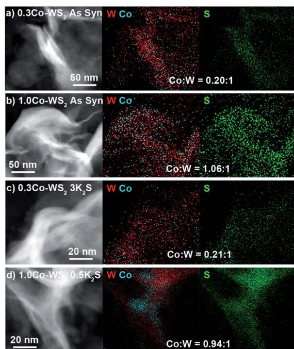
Fig. 2 STEM-EDS image and elemental maps of W, Co, and S for (a and b) as-synthesized 0.3Co and 1.0Co-WS<sub>2</sub> supported on C as well as (c and d) 0.3Co and 1.0Co-WS<sub>2</sub> after annealing with K<sub>2</sub>S.
