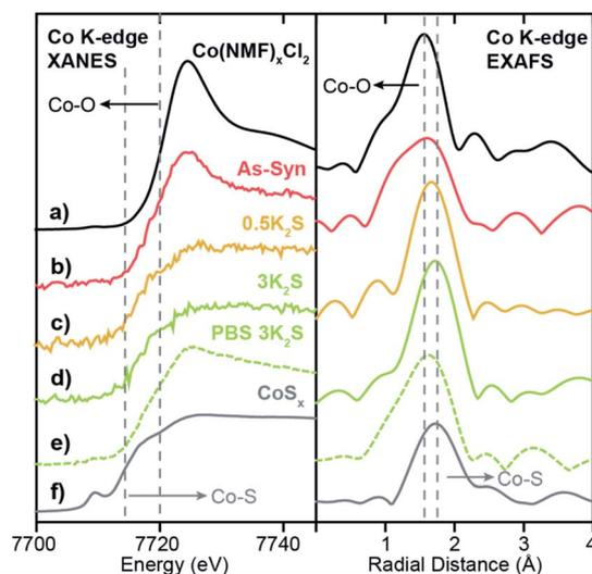
Fig. 4 Co K-edge XANES and EXAFS spectra for (a)  $Co(NMF)_xCl_2$ , (b) As-synthesized 0.3Co- $WS_2$ , (c) 0.3Co- $WS_2$  annealed with 0.5 equiv. of  $K_2S$ , (d) 0.3Co- $WS_2$  annealed with 3.0 equiv. of  $K_2S$ , (e) 0.3Co- $WS_2$  3 $K_2S$  immersed in 1 M PBS electrolyte, and (f) amorphous  $CoS_x$ . Dotted lines indicate the edge energies or scattering peaks for Co-O and Co-S coordination.
