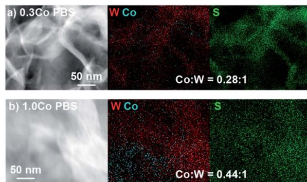
**Fig. 5** STEM-EDS image and elemental maps of W, Co, and S for (a) 0.3Co– $\text{WS}_2$  3 $\text{K}_2\text{S}$  and (b) 1.0Co– $\text{WS}_2$  3 $\text{K}_2\text{S}$  after treatment with PBS electrolyte.
