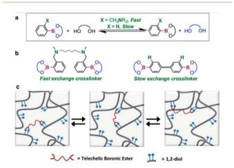
Fig. 4 (a) Kinetics of the exchange reaction of boronic esters according to their neighboring functional groups. (b) Transesterification reaction using boronic ester as a cross-linking agent. (c) Schematic of the boronic ester exchange reaction. Reproduced from ref. 55 with permission from the ACS.
