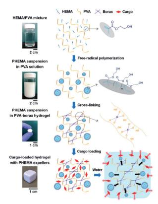
Fig. 25 Schematic of the drug release model and manufacturing method used to prepare a PVA-borax hydrogel embedding PHEMA in the micelles. Reproduced from ref. 120 with permission from the Wilev.
