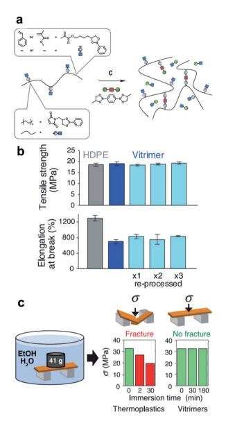
Fig. 7 (a) Synthetic scheme for various copolymers containing pendant dioxaborolanes (PS, PMMA, and HDPE). (b) Tensile properties of HDPE (gray column) and HDPE vitrimers (pristine: blue, reprocessed: light blue). (c) Environmental stress-cracking resistance of PS vitrimer. Reproduced from ref. 50 with permission from the AAAS.
