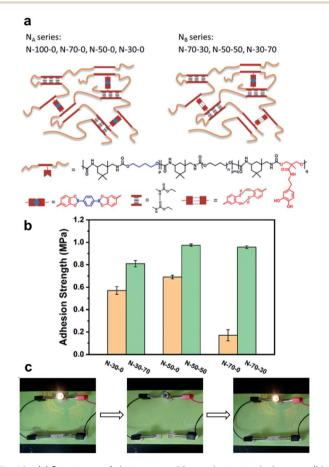
Fig. 10 (a) Structures of elastomers with pendent catechol groups (N<sub>A</sub>: no free catechol and N<sub>B</sub>: free catechol). (b) The adhesion strength of the elastomers. (c) Demonstration of the healing process for the silver/ elastomer composite with a light bulb. Reproduced from ref. 61 with permission from the ACS.
