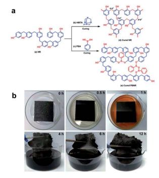
Fig. 8 (a) Synthetic scheme for the cross-linked NR with hexamethylenetetramine and the reprocessable PBNR. (b) The time-lapsed degradation process of the CF/PBNR composite laminate in ethanol at room temperature. Reproduced from ref. 51 with permission from the RSC.
