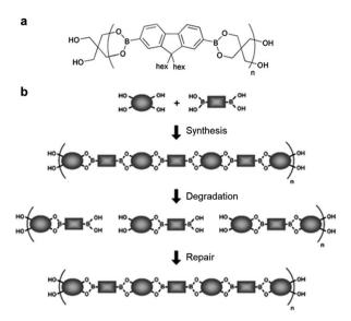
Fig. 3 (a) Chemical structure of poly(dioxaborolane). (b) Schematic representation of the synthesis, hydrolytic degradation, and selfhealing of poly(dioxaborolane). Reproduced from ref. 54 with permission from the RSC.
