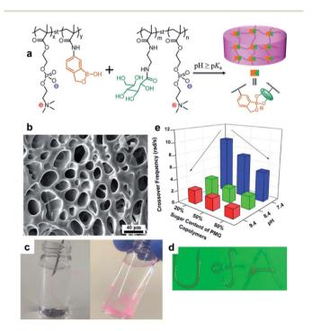
Fig. 26 (a) Synthesis of PMBG hydrogel using zwitterionic copolymers (PMB and PMG) bearing benzoxaborole and sugar pendant, respectively. (b) SEM image of the PMBG hydrogel. (c and d) Injectable properties of PMBG-50%-7.4. (e) Crossover frequency data. Reproduced from ref. 122 with permission from the ACS.
