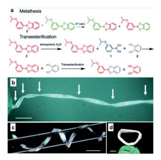
Fig. 11 (a) Mechanism for metathesis and transesterification reactions applied to self-healing organic crystals. Crystals of  $\bf 3$  twisted by  $1080^\circ$  (b), coiled around a glass capillary (c), and those with their two ends joined together to form a crystal ring (d) (Scale bars: (b) 1 mm; (c) 2 mm; (d) 1 mm). Reproduced from ref. 62 with permission from the RSC.
