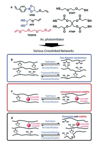
Fig. 5 (a) Cross-linked network of boronic ester prepared *via* photo-initiated thiol—ene click chemistry. Schematic of the boronic ester network exchange reaction in the presence of (b) free diol, (c) irreversible cross-linking, and (d) both free diol and irreversible cross-linking. Reproduced from ref. 57 with permission from the RSC.
