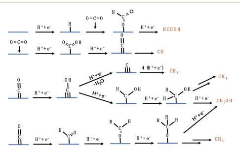
Fig. 4 The possible CO<sub>2</sub>RR pathways for C<sub>1</sub> products.
