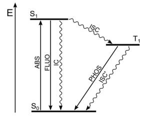
Fig. 2 Jablonski diagram for organic molecules with radiative (straight lines) and non-radiative processes (wavy lines).
