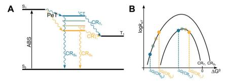
Fig. 4 Jablonski diagram illustrating the energies of the excited states involved in the SOCT-ISC mechanism (A) and related Marcus curve (B).
