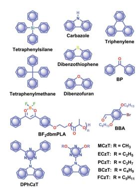
Scheme 1 Chemical structure of phosphors tetraphenylsilane, tetraphenylmethane, carbazole, dibenzothiophene, dibenzofuran, triphenylene, BP, BF $_2$ dbmPLA, BBA, DPhCzT, MCzT, ECzTPCzT, BCzT, and FCzT.
