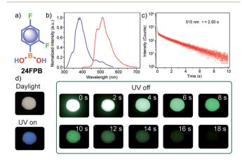
Fig. 3 (a) Chemical structure of 24FPB and (b) steady-state photoluminescence (blue line) and phosphorescence (red line) spectra of 24FPB. (c) Phosphorescence decay profile of the emission band at 515 nm. (d) Photographs of the 24FPB crystal taken at different time intervals before and after removing the excitation source (a 365 nm UV lamp). Reproduced with permission from ref. 80. Copyright 2019, WILEY-VCH.
