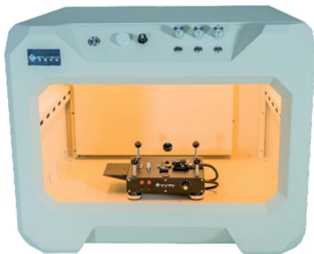
Fig. 3 Indoor PV testing setup as presented by, and reprinted with permission from Enlitech, ref. 36.
