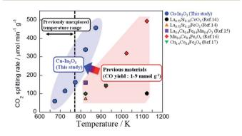
Fig. 2 Average  $CO_2$  splitting rates on the Cu-In mixed oxide (this study) and on various oxides in earlier reports.
