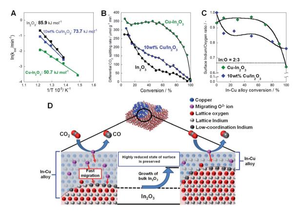
Fig. 6 Kinetics analysis of each oxide in re-oxidation steps. (A) Arrhenius plots for the oxidation of  $Cu-In_2O_3$  (derived from  $Cu_2In_2O_5$ ), 10 wt%  $Cu/In_2O_3$  and  $In_2O_3$ . (B) Dependence of differential  $CO_2$  splitting rate on conversion of oxides. (C) Surface In/O ratios on  $Cu-In_2O_3$  and 10 wt%  $Cu/In_2O_3$  during the re-oxidation step. (D) Presumed mechanism of  $CO_2$  splitting on the reduced  $Cu-In_2O_3$ .
