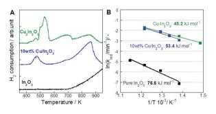
Fig. 5 Kinetics analysis of each oxide in the reduction step. (A)  $H_2$ -TPR profiles for  $Cu-In_2O_3$  (derived from  $Cu_2In_2O_5$ ), 10 wt%  $Cu/In_2O_3$  and  $In_2O_3$ . (B) Arrhenius plots for the reduction of  $Cu-In_2O_3$  (derived from  $Cu_2In_2O_5$ ), 10 wt%  $Cu/In_2O_3$  and  $In_2O_3$ .
