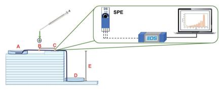
Fig. 7  $\mu$ FIA device configuration for LMG determination using amperometric detection (0.8 V), where A = electrolyte inlet, B = injection point, C = detection zone, D = electrolyte outlet and E = height of the device. The detector used consists of a carbon screen printed electrode (SPE) and the flow is directed through the system using the henequen fiber as a microchannel.
