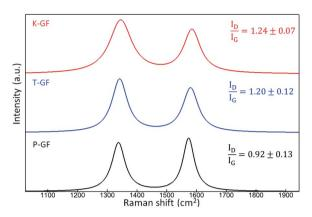
Fig. 4 Average Raman spectra indicating the D-band and G-band of P-GF, T-GF and K-GF electrodes. The average spectra are composed of five individual spectra which were fitted and smoothed using WITec Project.
