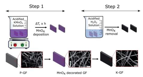
Fig. 1 Schematic diagram of the K-GF fabrication process. Step 1 involves the deposition of  $MnO_x$  layers onto the P-GF electrode surface using acidified  $KMnO_4$  solutions. Step 2 involves the removal of  $MnO_x$  layers using an acidified  $H_2O_2$  solution to produce the K-GF electrode. SEM images depict the fibre morphology during each stage of the fabrication process. The scale bars in each SEM image represent 50  $\mu$ m.
