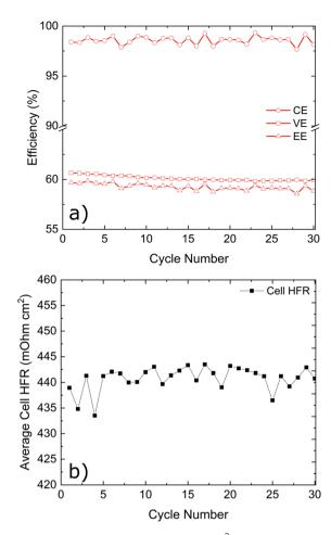
Fig. 7 K-GF electrode cycling at 400 mA cm $^{-2}$  for 30 cycles. (a) CE, EE and VE values for the K-GF electrode cycled at 400 mA cm $^{-2}$  for 30 cycles. (b) Average cell HFR values of the system during cycling.
