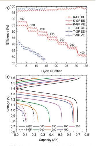
Fig. 6 (a) CE, EE and VE values of the T-GF and K-GF electrodes after cycling at multiple current densities from 100–400 mA cm $^{-2}$  in 1.6 M vanadium with 2 M  $\rm H_2SO_4$  and 100 mM  $\rm H_3PO_4$ . The P-GF electrode was unable to cycle at current densities higher than 40 mA cm $^{-2}$  and was therefore not included in this figure. (b) Voltage–capacity plot of the first cycle at each current density for the K-GF (solid) and T-GF (dashed) electrodes.
