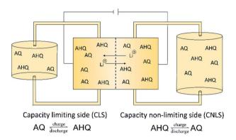
Fig. 1 Schematic representation of an unbalanced compositionally symmetric redox flow cell setup utilizing anthraquinone (AQ) as well as anthrahydroquinone (AHQ) and the representative half-cell reactions in the capacity limiting side (CLS) and non-limiting side (CLNS).
