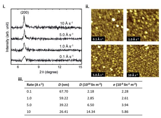
Fig. 5 (i) XRD pattern of CuPc thin-films, (ii) AFM images (1  $\mu$ m  $\times$  1  $\mu$ m) of CuPc thin-films, and (iii) crystal size (*D*), dislocation density (*d*) and lattice microstrain (e) of CuPc thin-films, deposited at various deposition rates. Adapted with permission from ref. 40. Copyright © 2012 Elsevier
