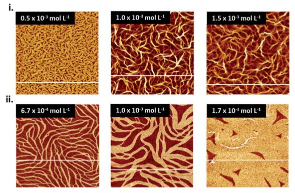
Fig. 8 AFM images ( $5 \mu m \times 5 \mu m$ ) of CuPc thin-films fabricated by (i) spin coating and (ii) dip coating at various concentrations of CuPc solution on SiO<sub>2</sub> substrates. (i) Adapted with permission from ref. 79. Copyright© 2020 the Authors under the Creative Commons Attribution Non-Commercial No Derivatives 4.0 License. (ii) Adapted with permission from ref. 80. Copyright© 2015 Elsevier B. V.
