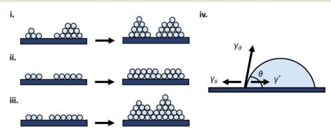
Fig. 3 Diagram of (i) island, (ii) layer-by-layer, (iii) SK thin-film growth, and (iv) relevant surface energies.
